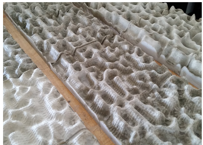
Figure 6. Prototype concrete relief panels cast from digitally milled molds. Oyster reefs were image sampled to create the panel form, with CNC milling creating the surface texture. Image credit: Author
