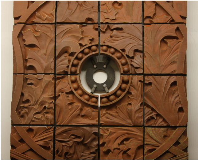
Figure 2. Terracotta detailing in the late 19th and early 20th Centuries ushered in a wave of architectural ornament in a variety of styles. Shown is a digitally fabricated replica of a cornice frieze detail from Louis Sullivan's Wainwright Building in St. Louis. Image credit: Author's design-build studio project.
