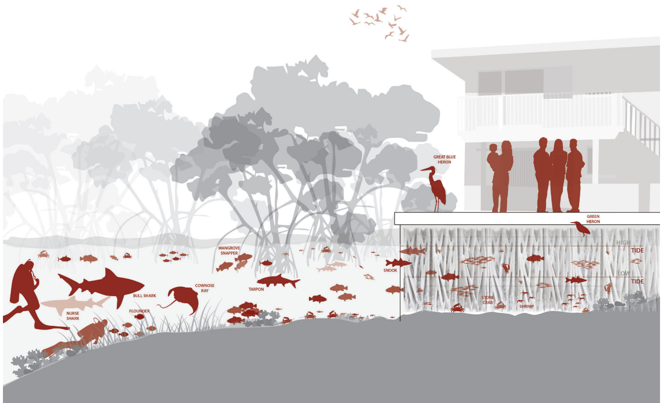
Figure 7. Biomimetic seawall concept utilizing digital design and manufacturing to create habitat and texture to support marine life. Image credit: Author.
